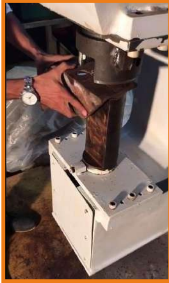
Angle punching with minimum back-mark on front side.
