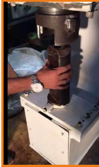
Die block could be rotated by hand for minimum back-mark on rear side of press.
