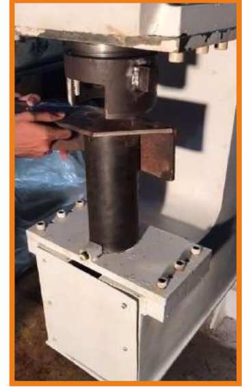
Punching Angle with minimum back-mark on rear side of press.
